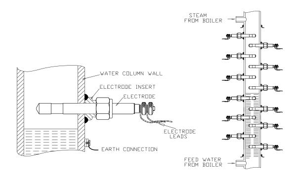
Figure 1.2 - Schematic of resistance measuring cell and electrodes
